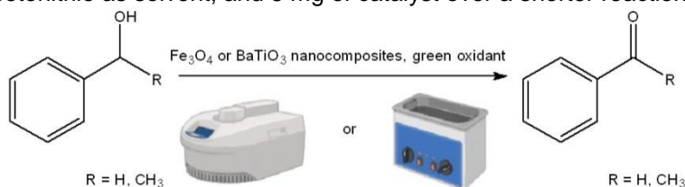
Scheme 1: Microwave or ultrasound irradiation assisted peroxidative oxidation of benzyl alcohols using Fe 3 O 4 and BaTiO 3 nanocomposites as heterogeneous catalysts.
