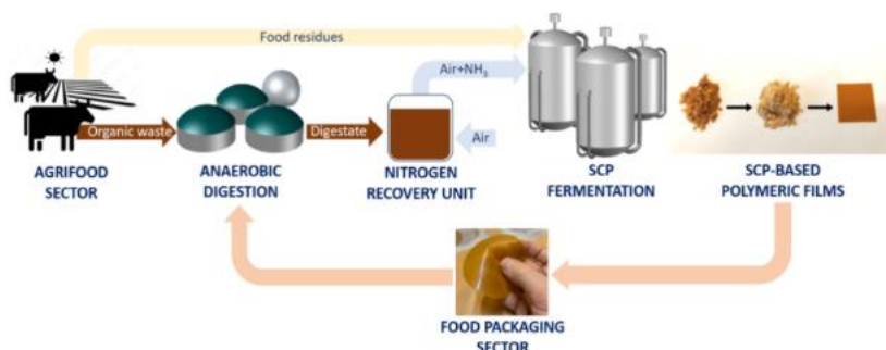
Figure 1. Integrated biorefinery scheme valorizing food residues and waste nitrogen into SCP-based biopolymers. The latter biopolymers can be used for food packaging applications and eventually be biodegraded and valorized through anaerobic digestion, targeting circular nutrient and energy recovery.
