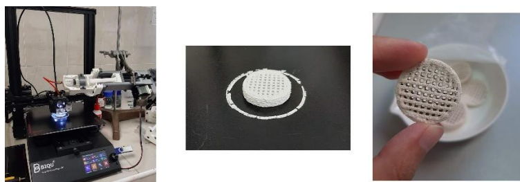
Figure 1. Stages of the monolith: during 3D printing, prior to calcination, and after calcination.
