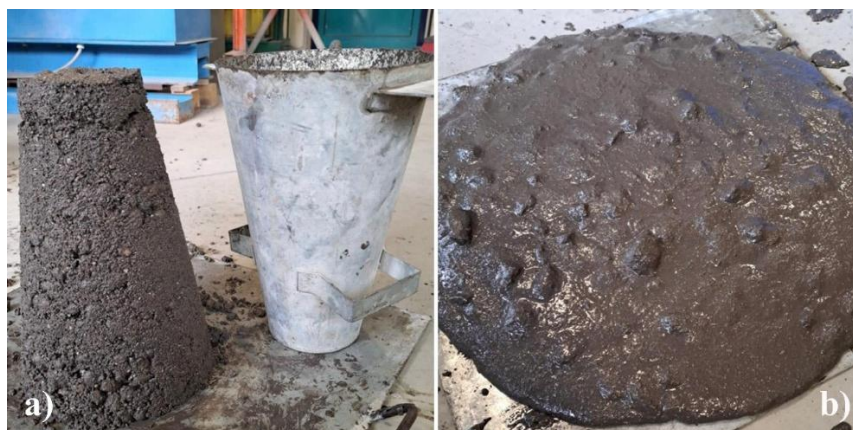
Figure 1. General view of the slump tests, showing the workability of the AFM2 (a) and control (b) pastes.
