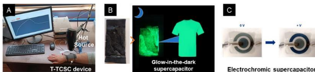
Fig. 1. A) Thermally-chargeable textile supercapacitor (T-TCSC), B) Glow-in-the-dark textile supercapacitor and (C) Electrochromic textile supercapacitor.
