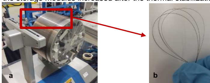
Fig.1. (a) PET-G/Lignin green fibers after the extrusion process; (b) PET-G/Lignin green fibers.
