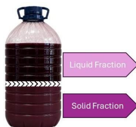
Figure 1. Natural decanting separation of the different red wine lees fractions.
